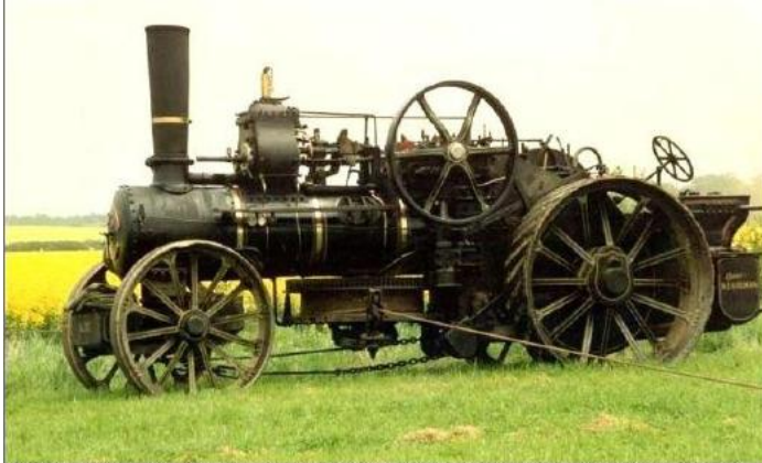
Steam plow of the type used in the sugar beet industry of the early 1900's. Note the drum and the cable strung under the belly of the behemoth. At the other end of the field would be another steam engine, each engine would be hooked to one end of the balance plow and would pull it back and forth.
