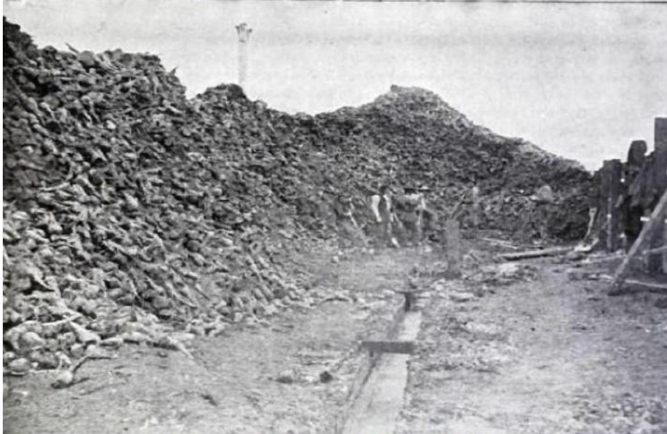
A sluiceway to carry beets to the factory in Alvarado, Calif.
