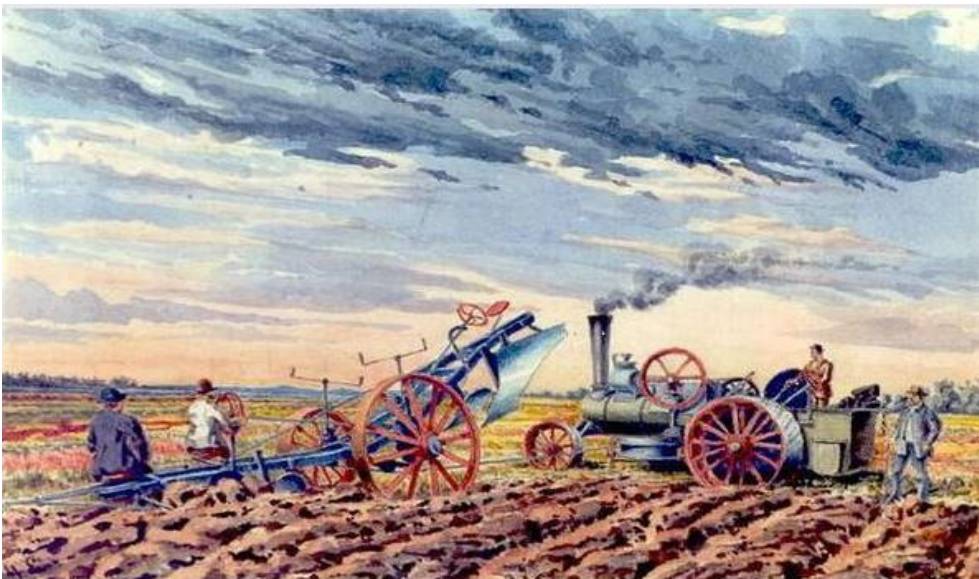
A drawing of a 1902 Fowler Steam Plough attached to a balance plough. Note the drum under the belly of the traction engine. The drum is loaded with a cable that can be released to free wheel in one direction and then locked as a take up spool to pull the balance plough forward. At the opposite end of the row is another steam plough attached to the rear of the plough. The balance plough is v-shaped with one end riding in the air as the plough is pulled forward. When the end of the rows are reached the rear gang is lowered and the steam plough at the opposite end of the field then pulls the plough forward.
