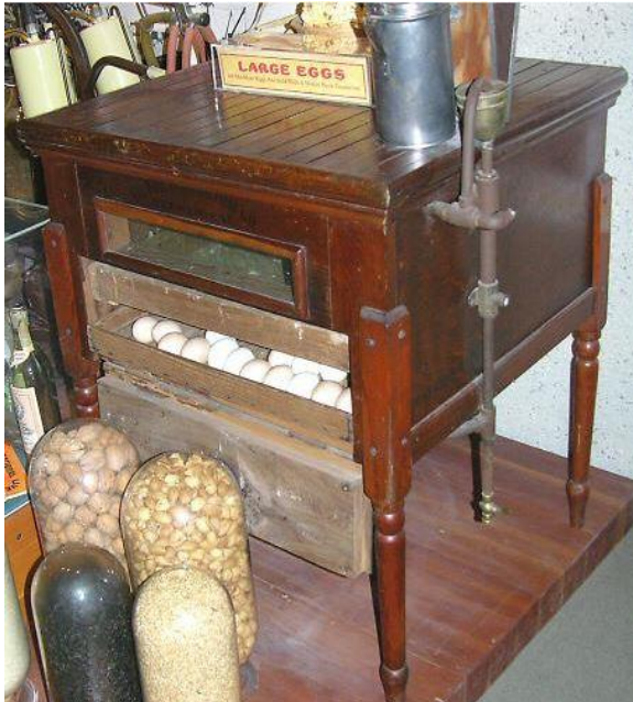
Wooden incubator for eggs, heated by wood and kerosene. Glass door in the front permits viewing of the eggs. Marked "Victor Incubator Co., Decoto Calif."
