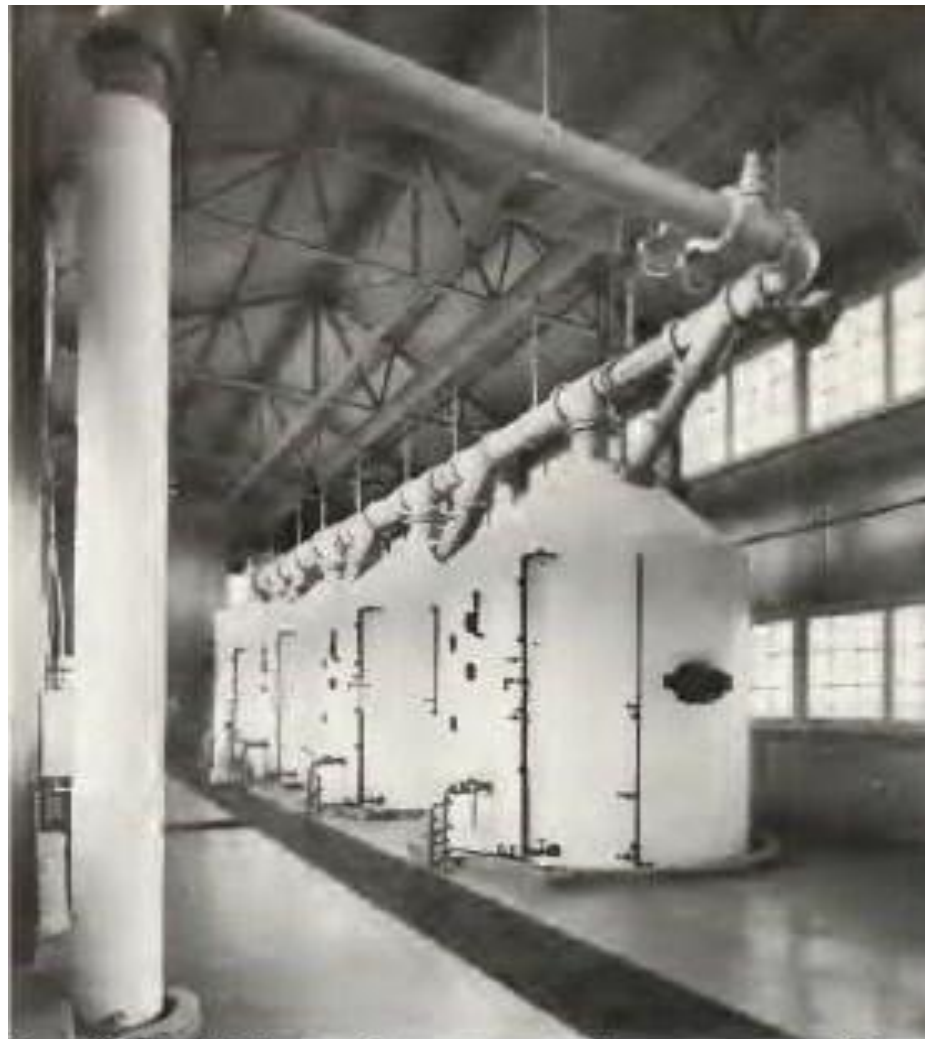
Leslie Salt Newark, evaporators, upper floor The refinery contains four Swenson basket type evaporators, three of which are used at a time in triple effect. As brine is boiled under vacuum within the evaporators, salt crystallizes in nearly perfect cubes.
