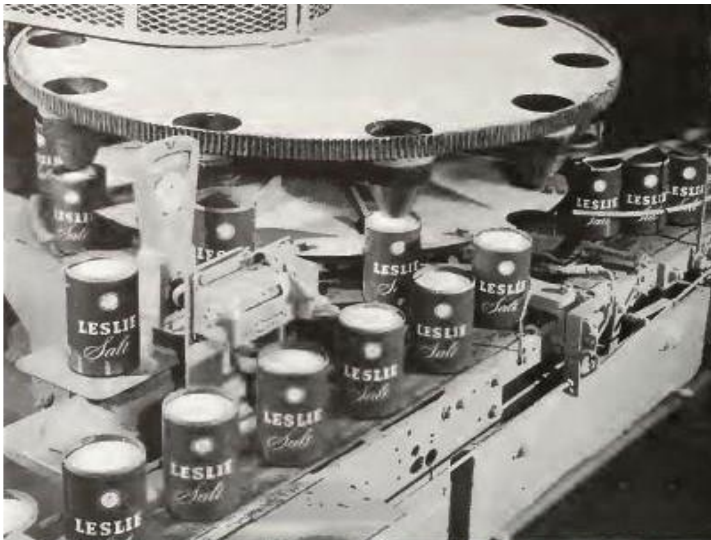
Leslie Salt Co., Newark: Filling and capping rounds at the Newark refinery. Machines fill the rounds with a measured amount of salt, cap them, label them, and prepare them for packing in boxes.
