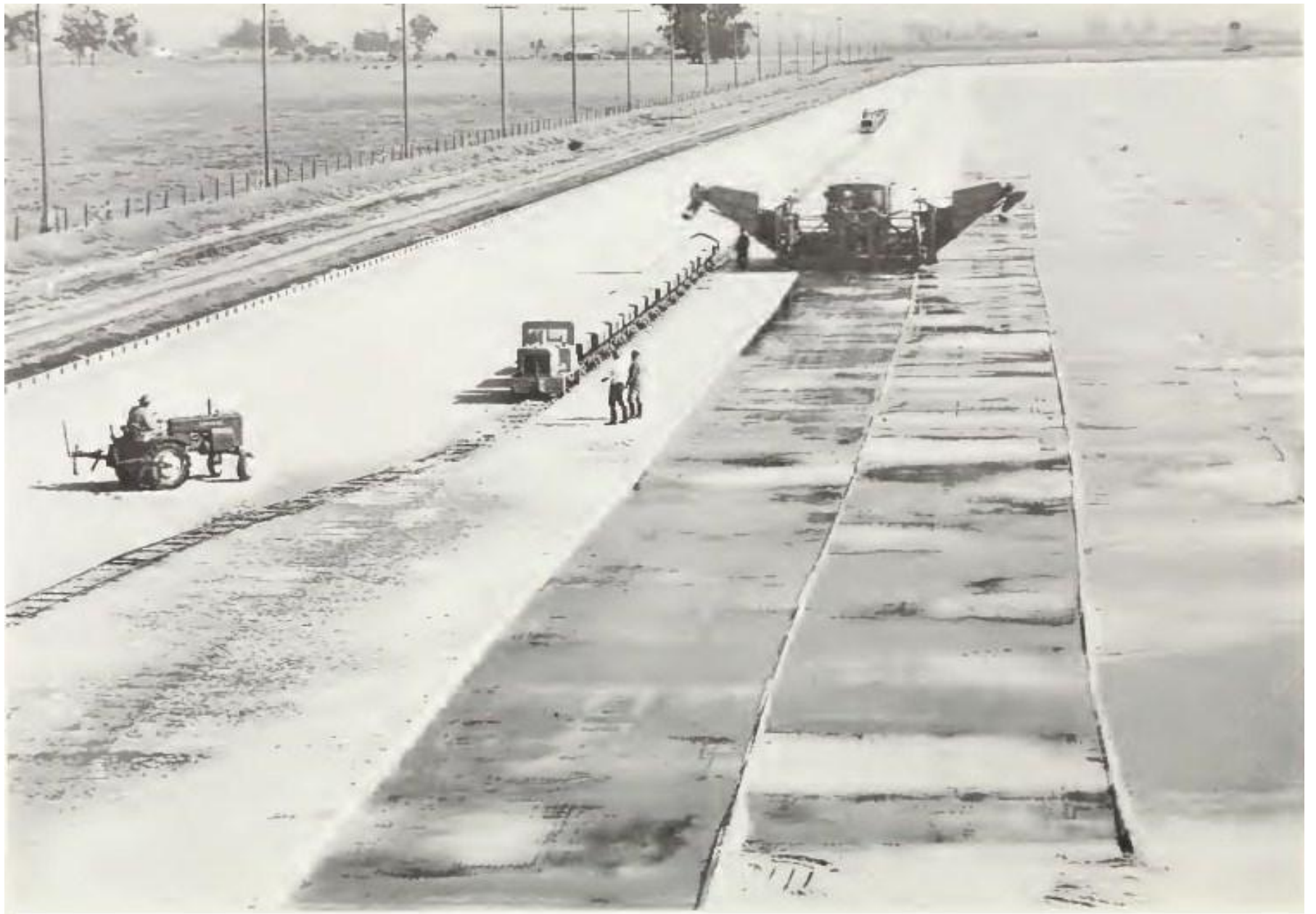
Leslie Salt harvesting machine in operation. Each harvesting machine is served by four trains of 12 to 14 cars. Permanent tracks are laid on the levees and temporary tracks on the salt.
