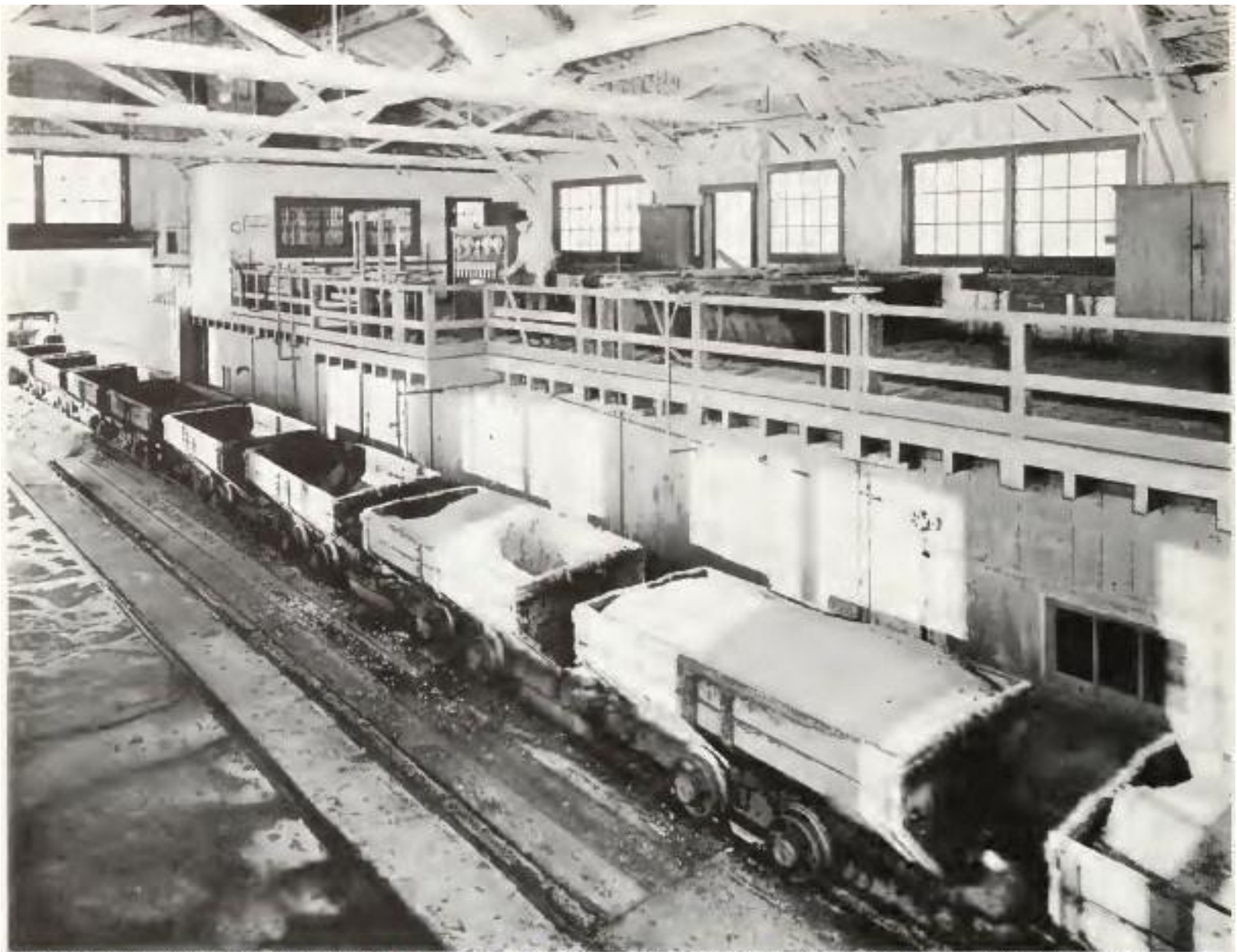
Leslie Salt Co., Newark: Dumping salt at the washer. The cars contents are discharged into rectangular brine filled pits beneath the tracks.
